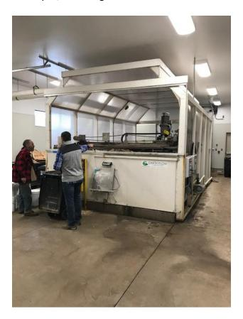
The unit cost \$144,000. It pumps heated air up through the compost mix, and also continuously agitates/stirs. The result is a reduction in process time per output batch to 4 weeks (vs. 3 months for aerated static pile).
