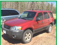
2007 Ford Escape; 144,046 miles. Projected repairs include front brakes, rear wheel bearings, alternator, exhaust pipe and flex tube, front ball joints.
